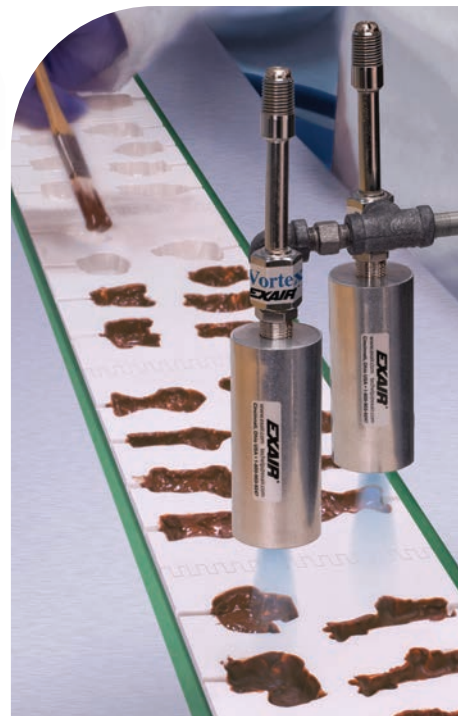
Dual Vortex Tubes rapidly cooling milk chocolate on a production line.
