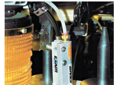
A Model 8103 3" (76mm) Gen4 Standard Ion Air Knife removes dust from computer hard disks prior to assembly.
