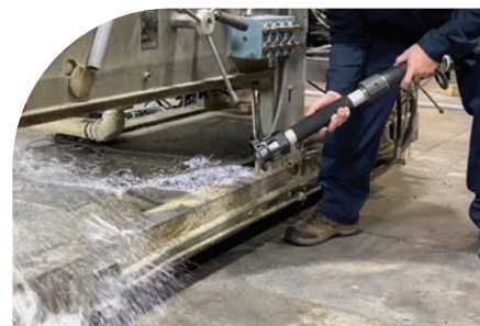
The TurboBlast Safety Air Gun blows away scrap paper trim.
